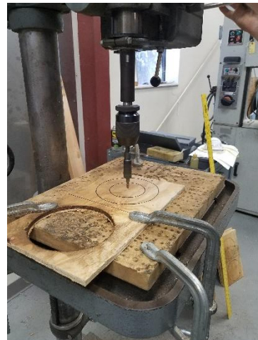
Figure 2 Drill press in use at the SDC
